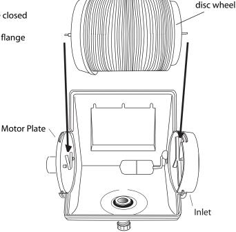
ensure tabs on inlet and motor plate fit into slots in lid flanges
